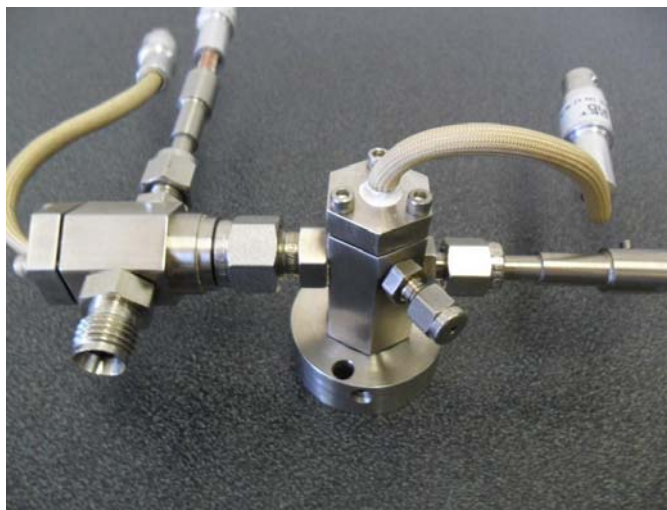
DET Tandem TID mounts on a Varian/Bruker FID/TSD detector base.
