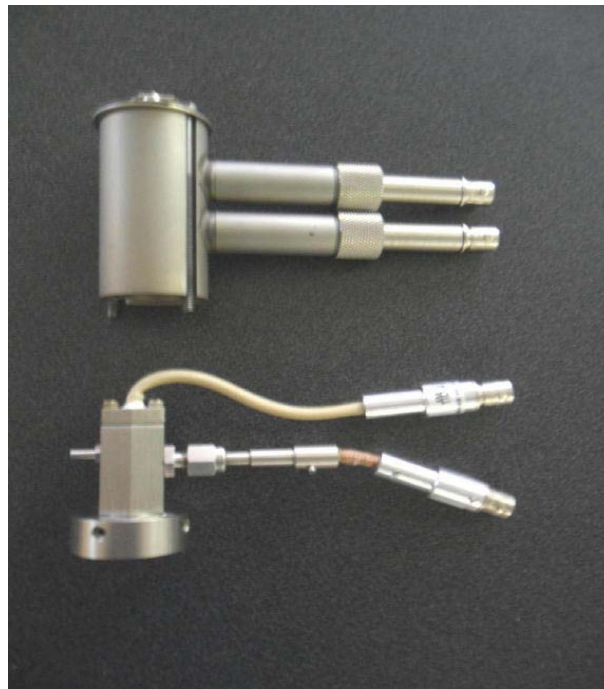
Comparison of Varian TSD Tower/Bead (Top) & DET NP/TID/FID Tower/Ion Source (Bottom). Top Mounting of DET Ion Source Allows Easy Access for Ion Source Replacements.
