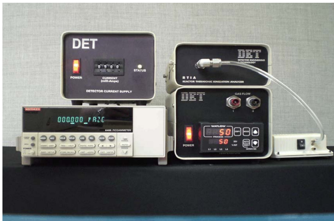
DET CURRENT SUPPLY, KEITHLEY ELECTROMETER, AND RTIA MODULE WITH AIR SAMPLE PUMP
