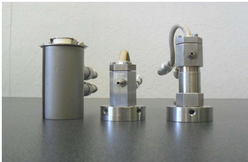
Varian/Bruker TSD on left, DET NPD/TID/FID in middle, DET Remote FID on right
