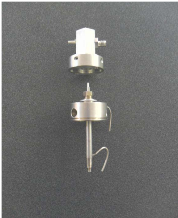
DET NP/TID/FID Tower Assembly & Ceramic Tipped Jet Custom Fit onto Varian FID/TSD Detector Base.
